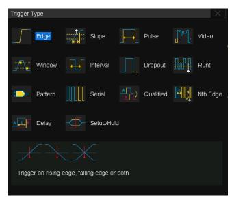
Edge, Slope, Pulse width, Video, Window, Runt, Interval, Dropout, Pattern, Qualified, Nth edge, Delay, Setup/Hold time, and serial trigger.
