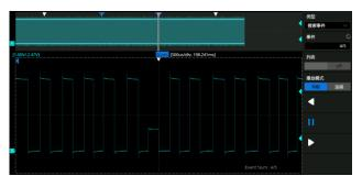
The oscilloscope can search events specified by the user in a frame. Events flagged by the Search can be recalled automatically using Navigate. It can also navigate by time (delay position) and history frames.
