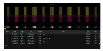
Display the decoded characters through the events list. Bus protocol information can be quickly and intuitively displayed in tabular form. I<sup>2</sup>C, SPI, UART, CAN, LIN, CAN FD, FlexRay are supported.
