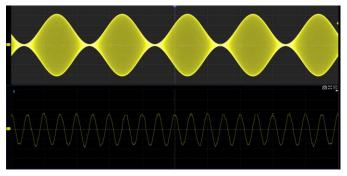
Using hardware-based Zoom technique and record length of up to 1 Gpts, users can select a slower timebase without compromising the sample rate, and then quickly zoom in to focus on the area of interest
