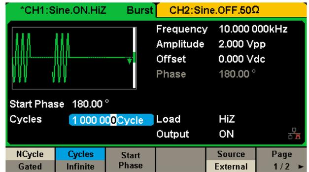
Two Burst modes, "N cycle" and "Gated". The Burst source can be configured as "Internal", "External" or "Manual".
