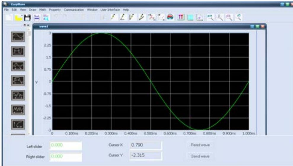
EasyWave is a powerful arbitrary waveform editing software program that supports several ways to generate arbitrary waveform such as manual drawing, line-drawing, equation-drawing, coordinate-drawing, etc. It is quite convenient for users to edit their own arbitrary waveforms through EasyWave.
