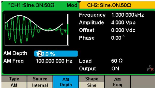
Multiple modulation types: AM, DSB-AM, FM, PM, FSK, ASK, PSK and PWM. The modulation source can be configured as "Internal" or "External".
