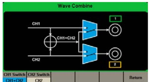
Capable of combining the waveforms of 2 channels from internal, providing more flexible tools to generate complex waveforms.
