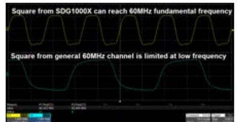
Benefiting from a special square-wave generating circuitry, the Square from the SDG1000X breaks the 60 MHz bandwidth barrier, reaching rise/fall times of less than 4.2 ns, and frequencies up to 60 MHz.
